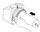
5. Remove the cooling drum seal from the rear of the drum.
