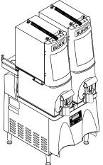
14. Install PAF unit onto platform and plug power cord into rear of platform. Plug platform power cord into proper outlet. (Refer to PAF manual for water connections)(Proceed to step 17)
