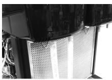
1. Connect syrup supply lines from BIB system. Connect water lines from source. NOTE: Connection points for these are marked on the rear of the motor cover.
