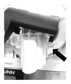
2. While slightly twisting the handle, spread the left side over the pivot pin to snap into place.
