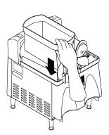
Slide the hopper(s) into place and push down until the hopper lock plunger snaps into place. For models without PAF, proceed to step 15.
