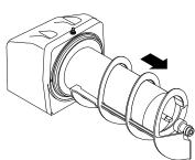
4. Pull the auger from the cooling drum.
