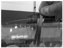
2. Install hoppers onto machine and slide probes onto hoppers into slots provided.
