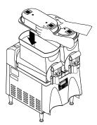
Set the lid(s) on the hopper(s). Lift slightly and slide back or front for filling.
