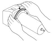
1. Install the seal(s) over the flange at 2. Align the auger shaft(s) with the the rear of the cooling drum(s) and press the seal(s) firmly into place as shown.
