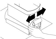
6. **Caution:** The faucet valve is under spring tension. Spread one side of the handle first, then the other and disconnect from the hopper.
