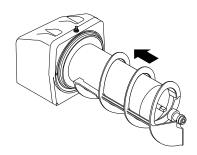
**9.** Align the auger shaft with the flat fin of the auger. Push the augers as far as they will go and rotate them so the flat fin is facing up.
