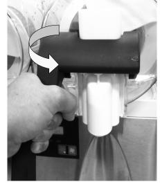
3. To remove the handle, twist in the same direction to free the handle from the left pivot pin, then slide off of the right pin.
