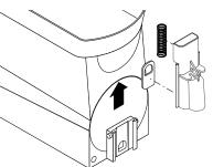
7. Carefully slide the faucet valve up to remove the spring and faucet seal. Extra care should be taken when handling the seal to prevent damage. Do not fold the seal as this will cause damage to the Teflon<sup>®</sup> sealing surface.
